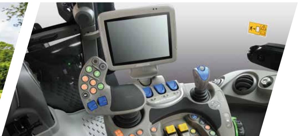
> Ergonomic joystick MaxCom with lift buttons, engine/transmission commands, button for gear management in the seat, two proportional hydraulic distributors and two assignable jolly buttons.
